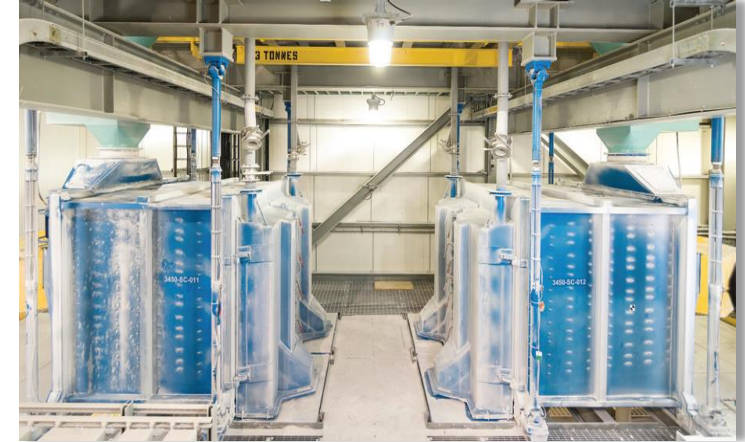
Fertilizer product loadout area; two Rotex Model MM5430-2 mineral separators
